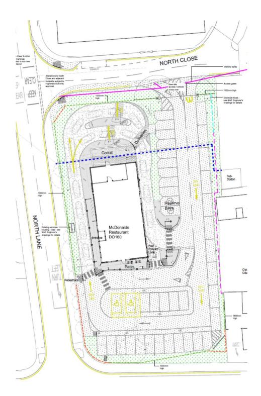
Figure 1: Approved Site Layout Plan 304 C: Note that the mini-roundabout at the junction of North Lane with North Close and Lower Newport Road is not shown on this plan since, at that time, the design was subject to approval by the Highway Authority (Hampshire County Council).
